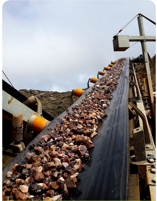
Rubber conveyor belt for rock loading
